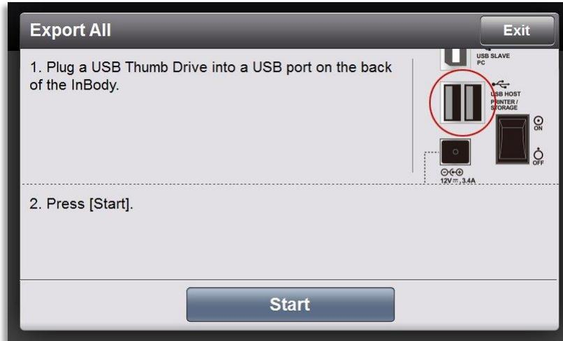
1. Plug the USB thumb drive to the USB port from the back of the unit.
